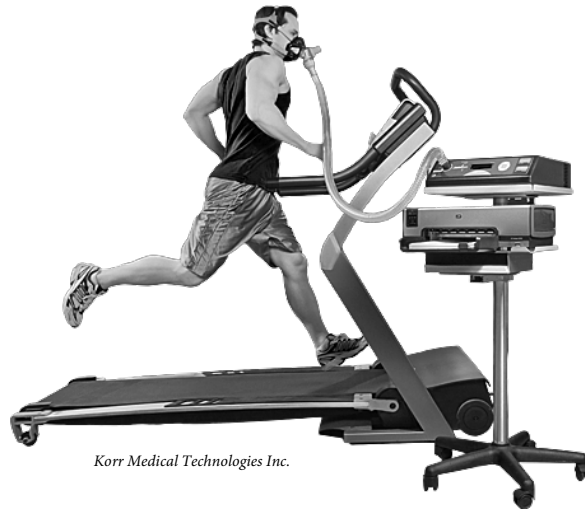
Figure 8.2. Apparatus for measuring oxygen consumption. This method is easier to do than the heat production method.
